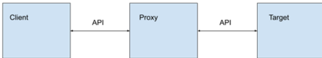
Figure 2.6 – The proxy object exposes the same API as the target
