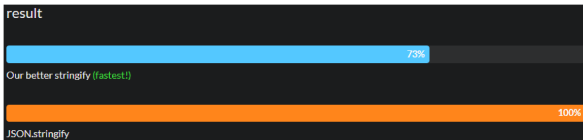
Figure 7.6 Performance difference between JSON.stringify and our method
