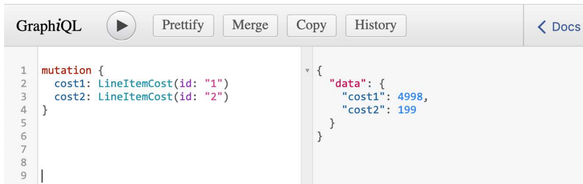
Figure 10.41: GraphiQL with LineItemCost aliased mutation queries for IDs "1" and "2"
